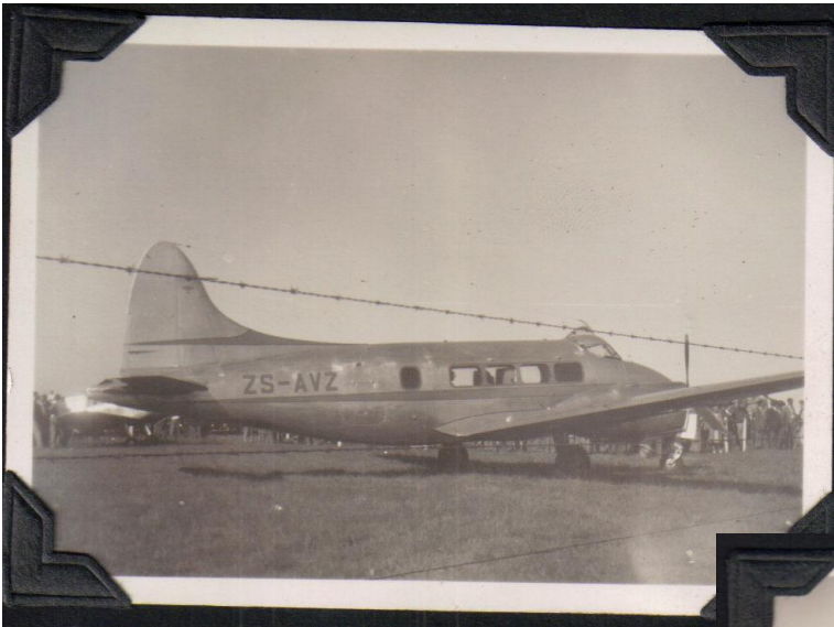
De Havilland Dove, with two Gypsy Queen Engines
