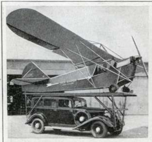
When alarm comes in, Oregon state police pursue fugitive criminals in this small plane, which takes off from platform mounted on top of a touring car as shown above.
